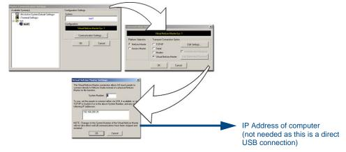
FIG. 36 Assigning Communication Settings for a Virtual Master
